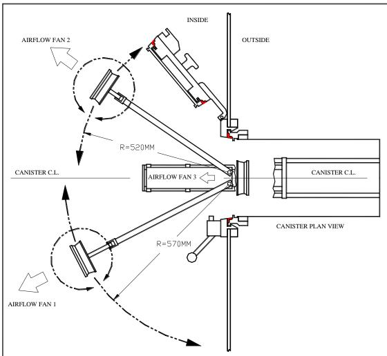
**Step 5**: Fan #1 and 2 are moved to the validated angular position and orientation. They are locked in position to assure of repeatability. Fan 3 is not adjustable.
