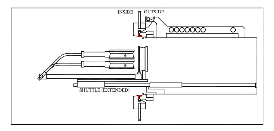
**Step 3**: The fan skid is pulled out of the NRC. The stroke is fixed and controlled by a hard stop.
