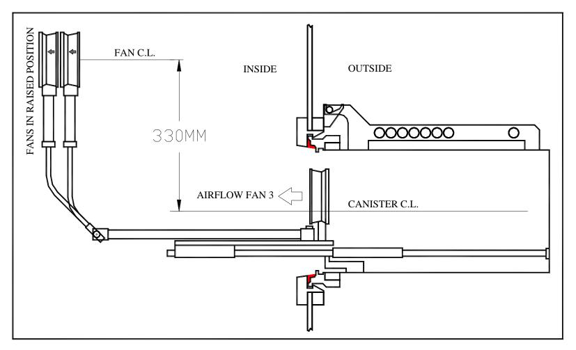
**Step 4**: Fans 1 and 2 are raised to the upright position. The extent of swing is controlled by hard stops to assure of positioning repeatability
