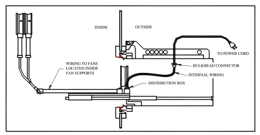
**Description:** The power cord penetrates the canister body via a leak tight bulkhead connector. The wires are routed to a distribution box where wiring to the individual fans is started. Wires to the movable fans is routed within the mounting arms.
