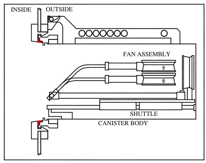
Step 2: The Alpha/Beta door is opened to gain access to the fan skid inside the NRC
