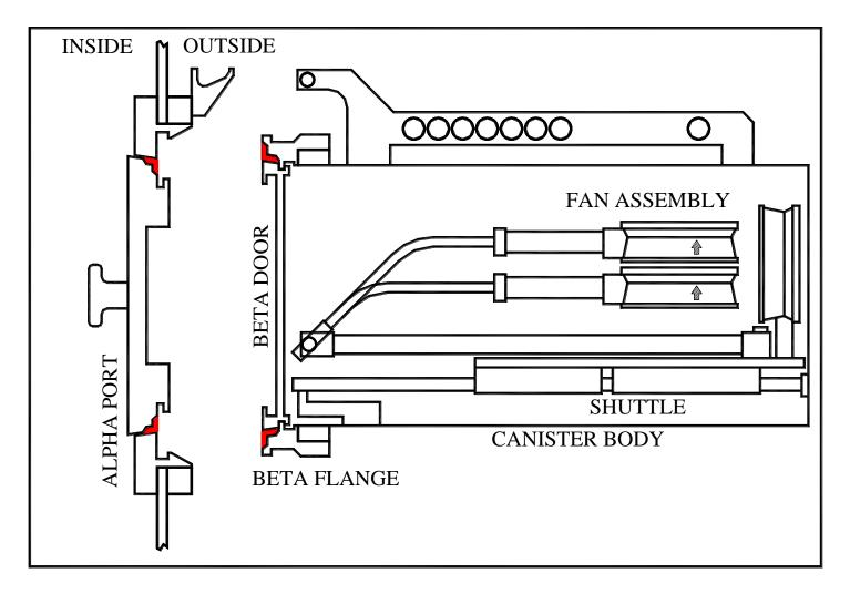
Step 1: The Air Mixing Module NRC is docked to the Alpha port of the barrier isolator
