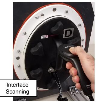
Note: Scanning of both the gloveport and the interface and automatically checking the validity of both scans assures the elimination of operator mistakes
