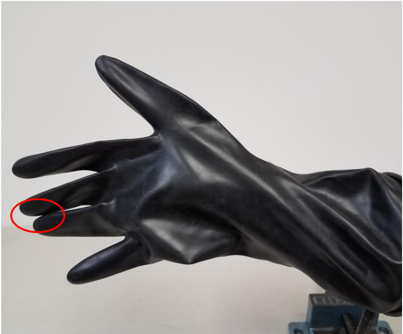
Figure 8 - Two finger support - (Thumb and little finger)
