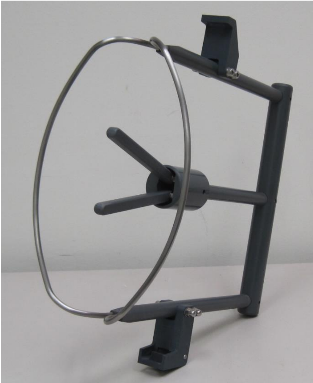
Figure 1 - Typical glove support design (two finger unit shown)
